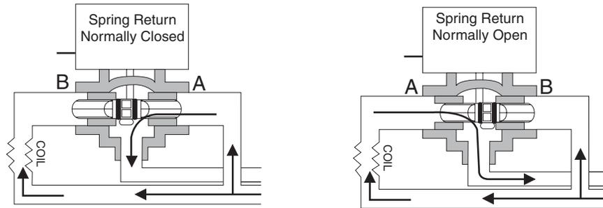
Figure-8 Three-Way Spring Return Valves.
